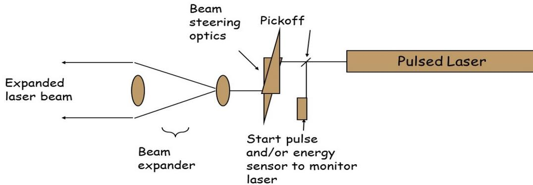
Figure 2. Simple diagram of ceilometer transmitter.
