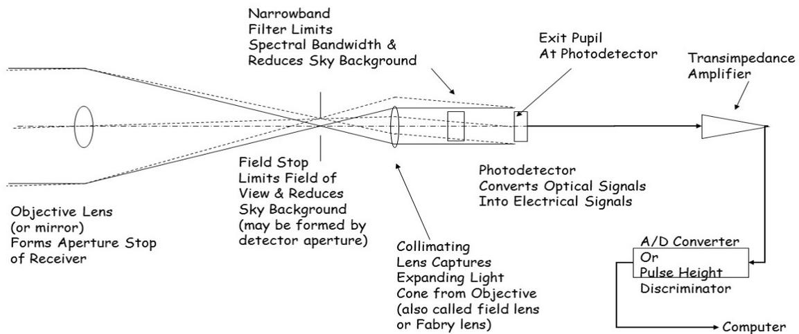
Figure 3. Simple diagram of ceilometer receiver.
