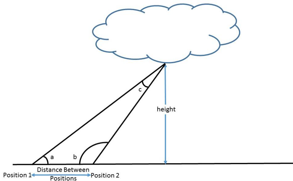
Figure 1. Illustration of height measurement using triangulation. If angles  $a$ , and  $b$  are known, as well as the distance between positions, then trigonometry can be used to obtain the cloud height ( $h$ ).
